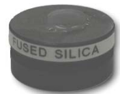
Fused-silica standard specimen on hardened, ground steel specimen mount.
