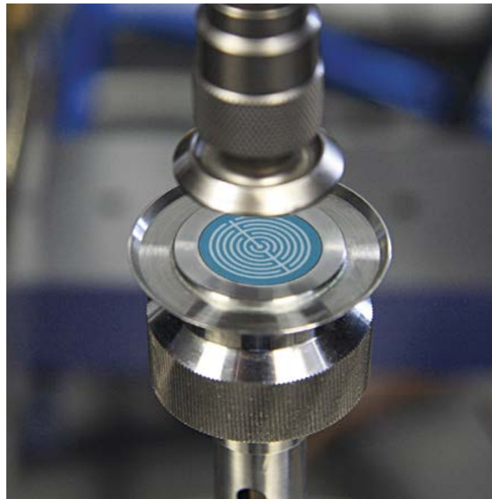
DEA 288 Ionic with reusable TMCc sensor (comb sensor with 0.5-mm electrode spacing), integrated in a MARS III Rheometer (plate-plate, gap >0.6 mm)
