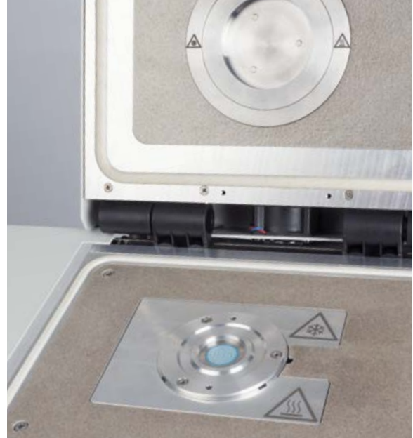
DEA furnace with installed Coated Tool Mountable Comb Electrode
