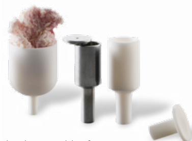
Large beaker crucibles for high-volume TGA tests
