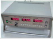
HMS 2000 Hall Effect system 10nA ~ 20mA Auto/Manual alternatively
