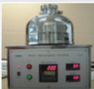
RTA 2000 Controlled by PC s/w. RT ~ 1200 °C 1000 °C /40seconds
