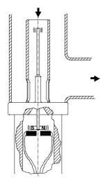
The vibration amplitude varies according to the product's viscosity where the rod is immersed
