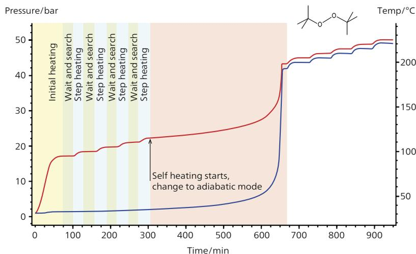
HWS test on 20% di-tert-butyl-peroxide (DTBP) in toluene. For the investigation of self-heating behavior, the measurement can include isothermal segments or temperature ramps.
