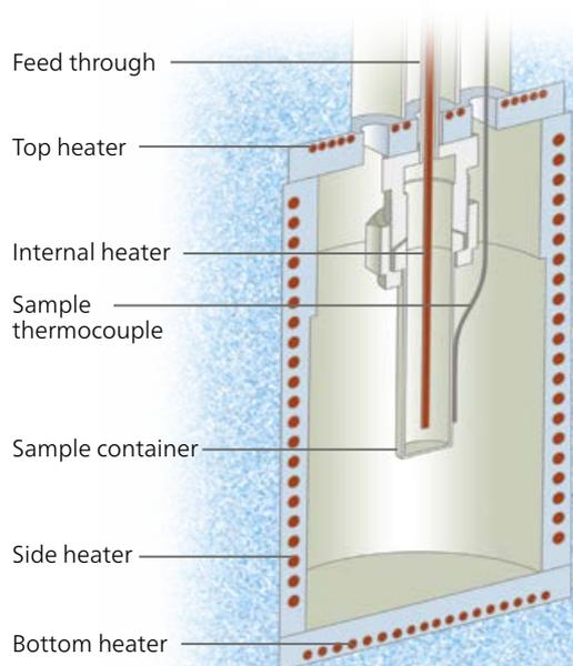
ARC Module with optional VariPhi® (internal heater)
