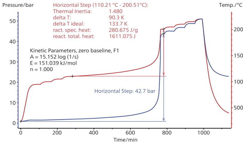
Heat-Wait-Search test on 5.74 g of 20% di-tert-butyl-peroxide (DTBP) in toluene in a spherical titanium vessel (mass 10.028 g); exothermal threshold 0.02 K/min, thermal inertia: 1.48
