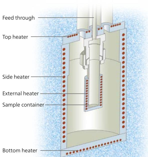
Scanning Module with external heater
