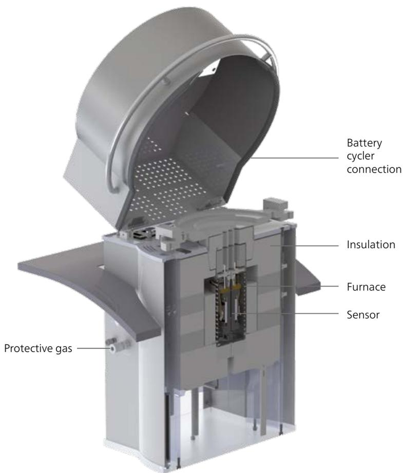
Cross section of the Coin Cell Module
