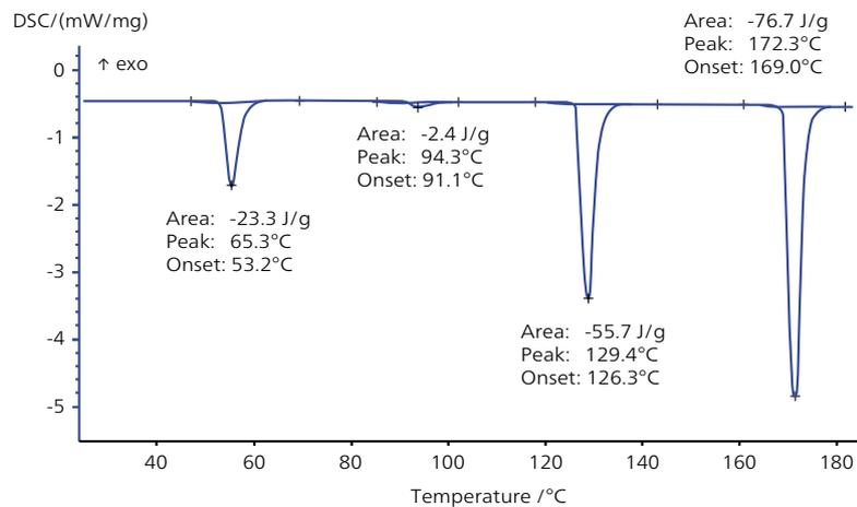
DSC 204 F1 Phoenix® measurement on  $\text{NH}_4\text{NO}_3$  up to 200°C. The sample undergoes three endothermic solid-solid phase transitions followed by melting at 169°C (onset). With increasing temperature after melting, the material will thermally decompose.
