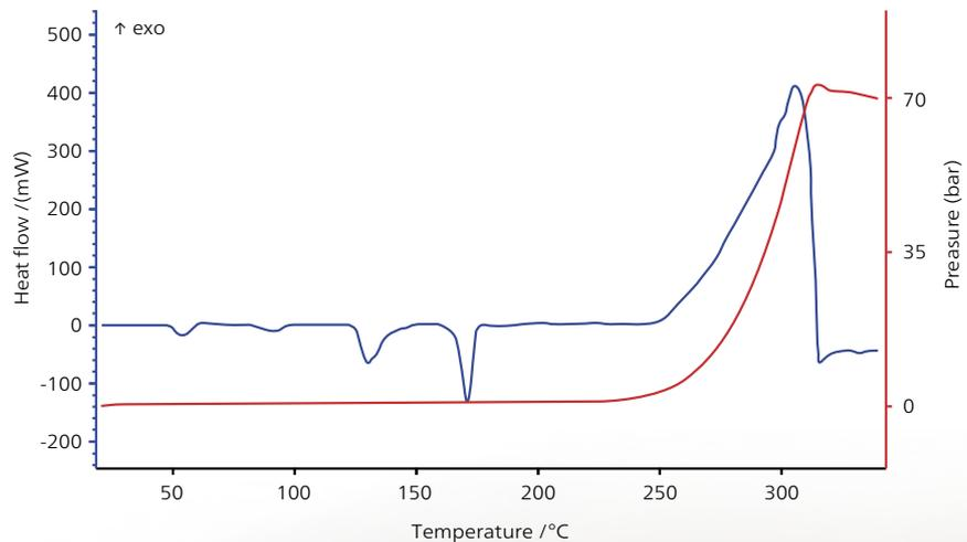
ARC Module with VariPhi® plot of  $\text{NH}_4\text{NO}_3$  with heat flow and pressure versus time
